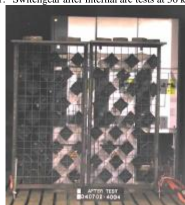
FIGURE 1: "Switchgear after internal arc tests at 36 kV/25 kA/1s"
