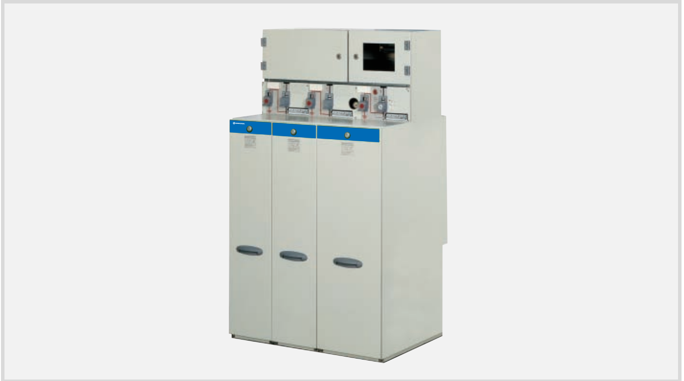
Three panel switchgear, Type GA2K1LSF250, with two cable feeder load-break switch panels and one feeder circuit-breaker panel, including relay/control compartment on the top.
