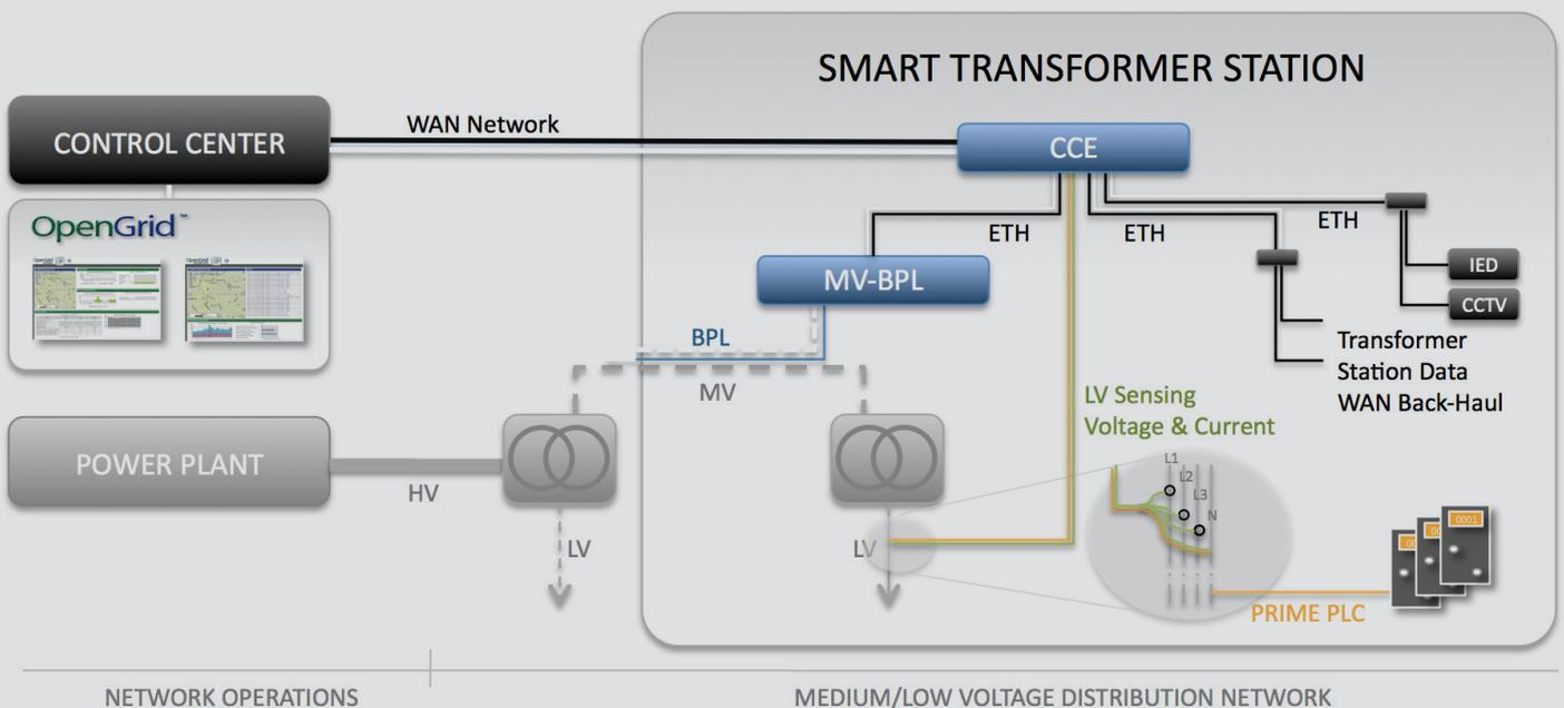
Figure 2 – Schematic of smart transformer station
