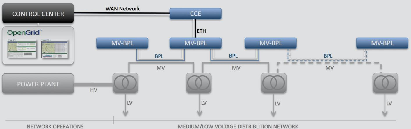
Figure 1 – Schematic of Electrica's MV connections
