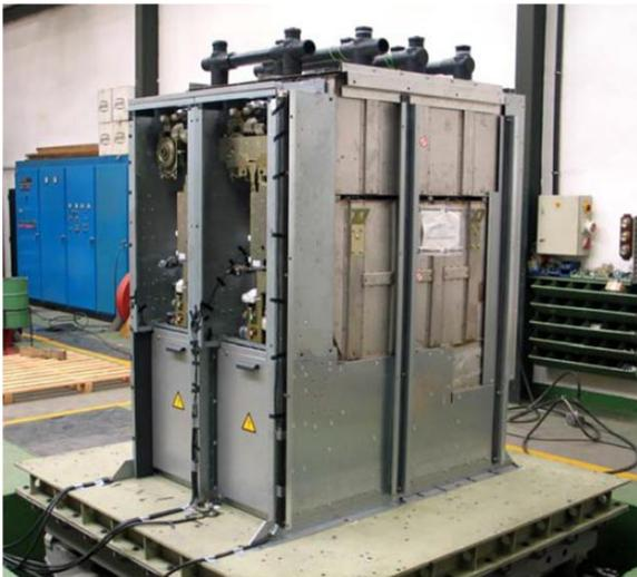
The tests have been performed on a shake-table provided with a "bi-axial independent" action, and powered by two hydraulic actuators, a vertical one and a horizontal one, with a variable frequency and amplitude, independent from each other.
