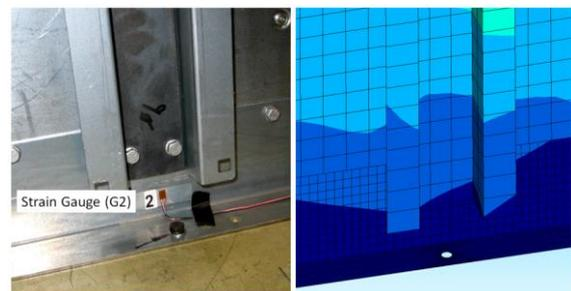
As stated before, to obtain accurate strain and stress results it is vital to assess that the mesh quality is enough to ensure the convergence of results, especially around the strain gauge position. Moreover, if the location of the strain gauges is close to an area where the gradient changes abruptly it is of the utmost importance to know the precise position of the gauges over the equipment.
