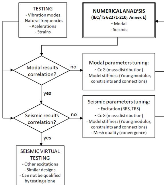
The complete seismic assessment methodology is applied over ORMAZABAL's CPG.1 gas insulated, single and double busbar cubicle for primary distribution.
