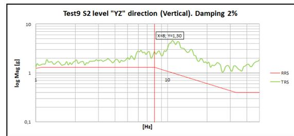
Besides, in order to achieve a good correlation, the excitation of the simulation model should be the TRS, enveloping the RRS, because it is the actual seismic load when the physical test is performed (see Picture 5).
