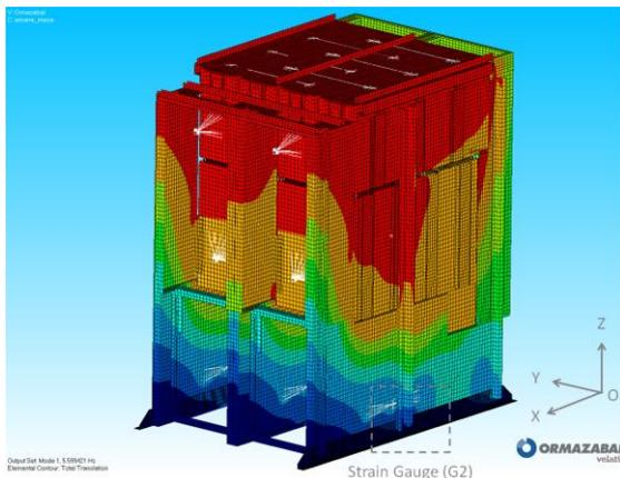
2) Modal results: For the analyzed equipment, the first two modes have an important proportion of mass involved. These two modes are: Mode 1 at 5.60Hz (95% mass in side-to-side OY direction) and Mode 2 at 20.06Hz (55% mass in front-to-back OX direction)<sup>2</sup>. The former natural frequencies and mode shapes match with those obtained in the resonance search tests.
