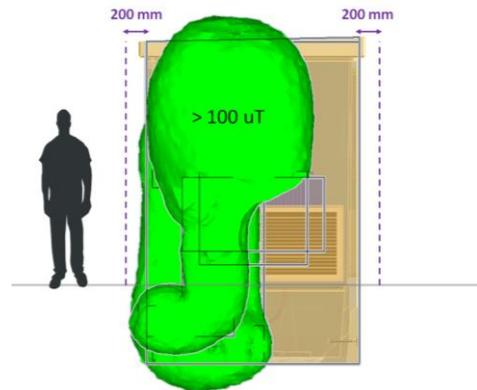
Picture 6. TS top view (Magnetic field over 100 $\mu$ T).
