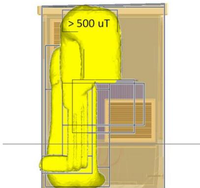
Picture 9. TS top view (Magnetic field over 500 $\mu$ T).
