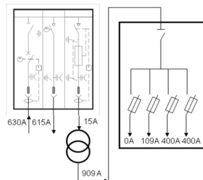
In the case of the LV board each phase can deliver 4 LV outputs each one limited to 400A by a fuse. In order to simulate the worst case scenario the outputs excitation has been set as follows (from left to right): 0A, 109A, 400A, 400A. The latter being the closest to the concrete enclosure.
